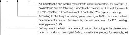
indicates maze-type sealing and 02 indicates comma-type sealing. H indicates a Herman product and SS is the abbreviation of skirt seal.
